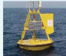
Diamond Shoals Data Buoy installed in Monitor sanctuary, providing real-time water and weather data.
