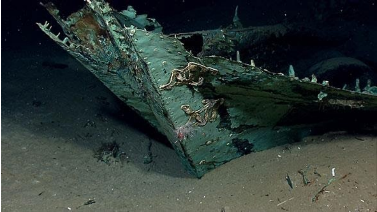
Figure E.4. Copper sheathing covers the stern post of Monterrey A. Photo: NOAA Okeanos Explorer Program
