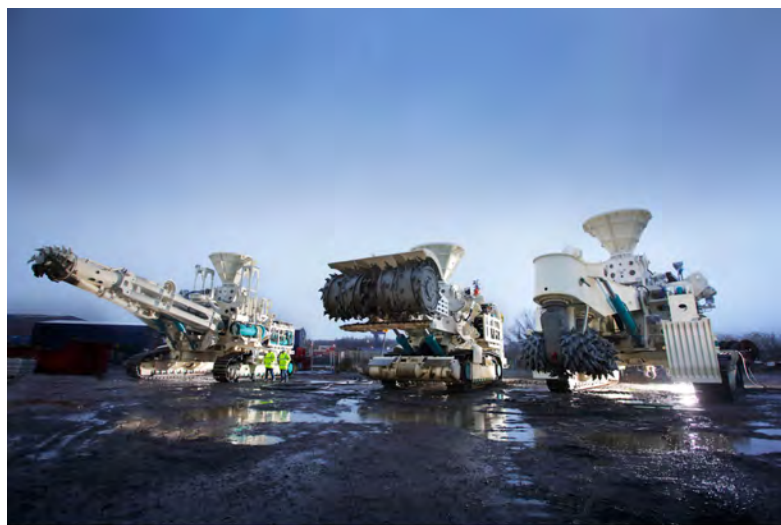
Figure 4. Deep-sea mining machines, two for cutting and one for collection. For scale, note the people in yellow jackets next to the machine on the left. (Photo credit: Nautilus Minerals)
