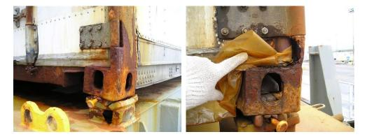
Figure 8. Container corner posts and fittings in unsatisfactory condition. Figures from AIMU 2008.
