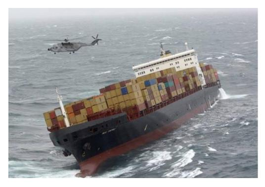
Figure 6. The *MSC Napoli*, which broke apart in January 2007 in the English Channel. MAIB investigation determined that 20% of the containers were overweight. Photo from AIMU 2008.
