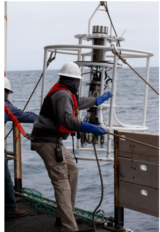
A crew member from the NOAA ship Bell M. Shimada deploys a conductivity, temperature, and depth (CTD) sensor. Repeated measurements of the water column can establish a record of change. Photo: Chad King/NOAA
