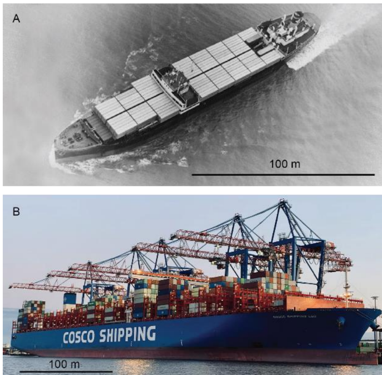
Figure 1. A size comparison of (A) the original container ship Ideal-X in 1956 and (B) the modern container ship COSCO Shipping Leo in 2020. Ideal-X was photographed during its inaugural voyage as a container ship with a maximum capacity of 58 containers on board. In photo B, COSCO Shipping Leo was loaded with a fraction of its 15,200 twenty-foot equivalent unit capacity (7,600 full size containers). Photos: (A) United States Merchant Maritime Academy; (B) Jacob Meissner/Unsplash
