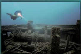
An underwater archaeologist inspects the ship's windows. A window is used to raise and lower the anchors.
